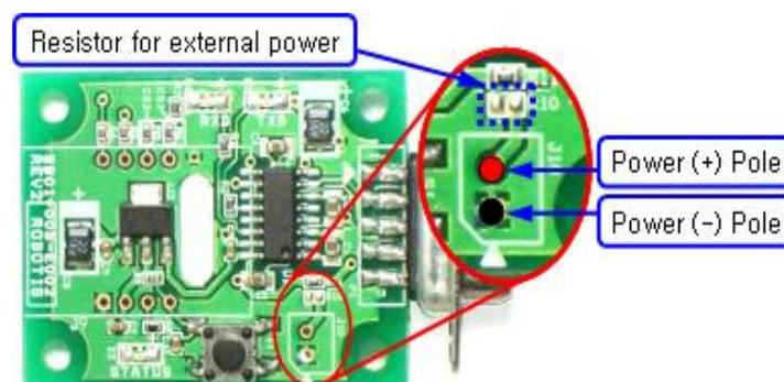
**Zero ohm resistor** must be attached or **connected by soldering** on the location of **resistor for external power** to supply the external power.
